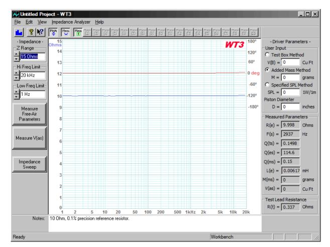
Here is a typical result when measuring a 10 Ohm resistor:
